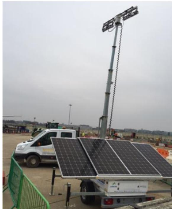
*Ferrovial Agroman UK has installed 100% solar powered lighting towers at sites across the airport.*
