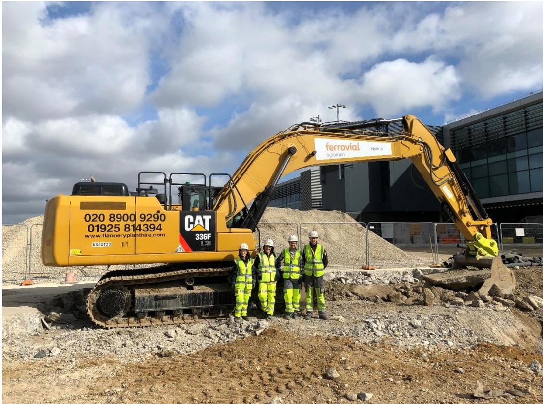
*Ferrovial's hydraulic-hybrid excavator uses 66 tons less CO<sub>2</sub> than the standard model over the course of a year. This is the equivalent of taking 20 diesel cars off the road.*
