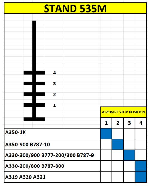
These boards will be located at the head of stand by the Stand Entry Guidance control panel.
