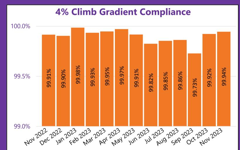
METRIC: A departing aircraft will maintain a minimum climb gradient of 4% measured between 1000ft and 4000ft.
