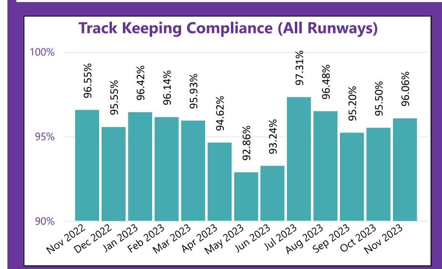
**METRIC:** Aircraft shall be deemed on track when it remains within a swathe 1.5km either side of the Standard Instrument Departure ideal centre line.
