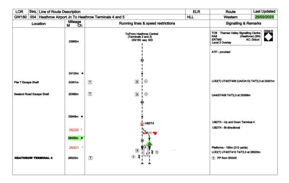
The changes made in the marked-up diagram above reflect the change in speed from 30mph to 20mph at 26220m on the Terminal 4 Platform 1 Line, together with the addition of a new speed board.
