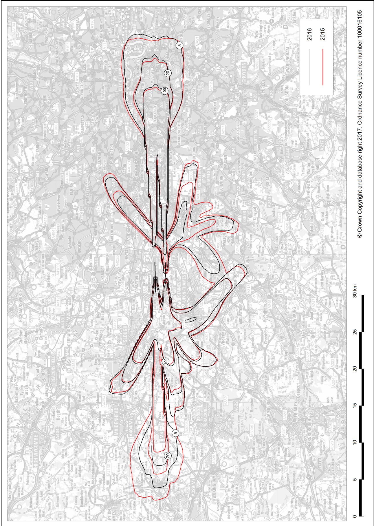
Figure B10 Heathrow 2016 and 2015 average summer day overflight contours (assuming 48.5 degree elevation angle)
